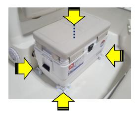
2. Remove chocks and cooler/cargo. Mark remaining holes for bases, install bases using screws included (!!Care should be taken for proper clearance under deck, as well as the proper drilling of pilot holes and sealant if necessary)
